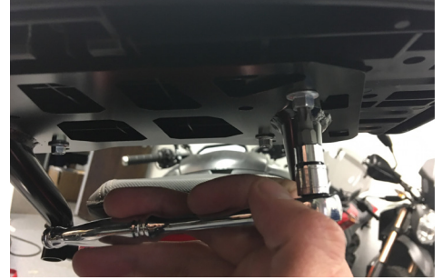
Figure 23. Mount The SHAD Adapter Plate (below)
