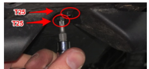
Figure 16. Turn Signal Support Bracket and Cover Attachment
