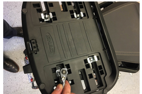
Figure 24. Mount The SHAD Adapter Plate (above)
