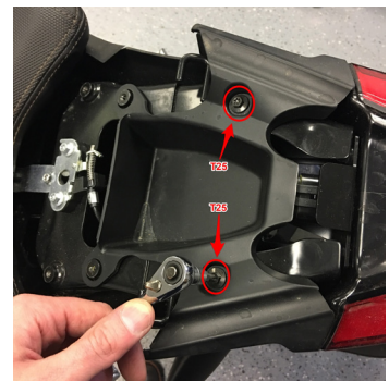
Figure 5. Seat Tray Removal
