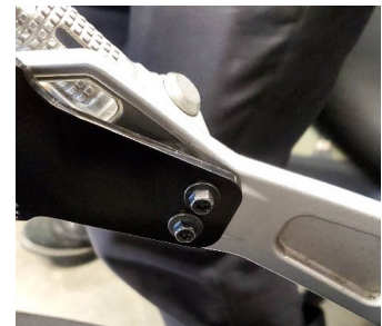
Figure 12. Side Case Support Secured To Rear Set
