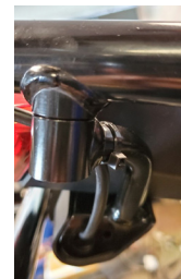
Figure 20. Secure Top Rack Turn Signal Support
