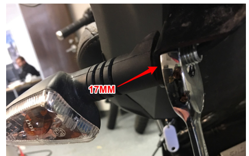
Figure 4. Turn Signals Detached
