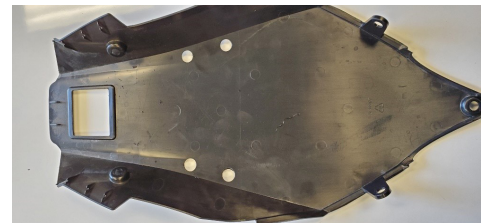
Figure 10. Tail Trunk Pan With Drilled Holes
