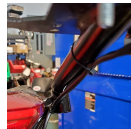
Figure 22. Route And Secure Turn Signal Wires
