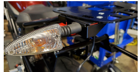
Figure 21. Attach Indicator Support To Top Rack
